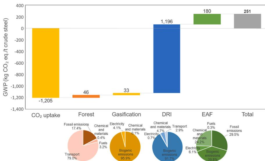
Fig. 5. Cradle-to-gate GWP of crude steel production via biosyngas-DRI-EAF route without CO<sub>2</sub> storage. The GWP is presented per subsystem, each includes both direct and indirect emissions. The pie charts show the percentage of emissions contribution.
