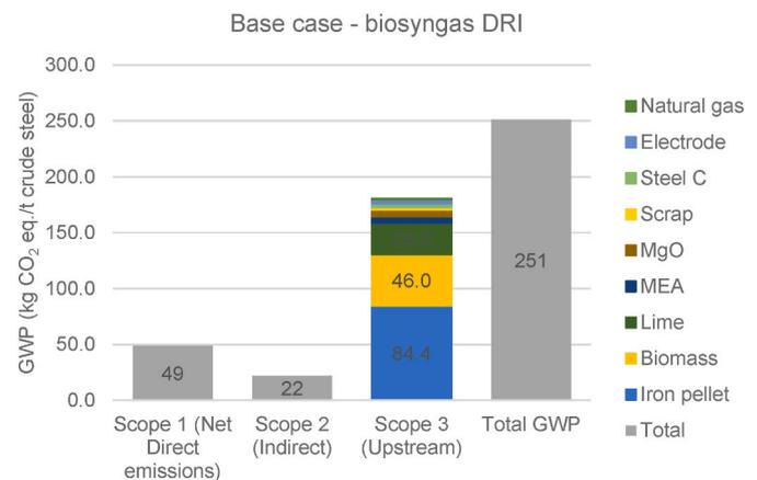
**Fig. 4.** Cradle-to-gate GWP of crude steel production via biosyngas-DRI-EAF route without CO<sub>2</sub> storage. Scope 1 refers to net direct emissions, including biogenic emissions, fossil emissions and CO<sub>2</sub> uptake by the plant. Scope 2 emissions are indirect GHG emissions associated with the purchase of electricity. Scope 3 emissions are all indirect emissions (emissions from the extraction, processing and transportation of raw materials), not included in Scope 2.
