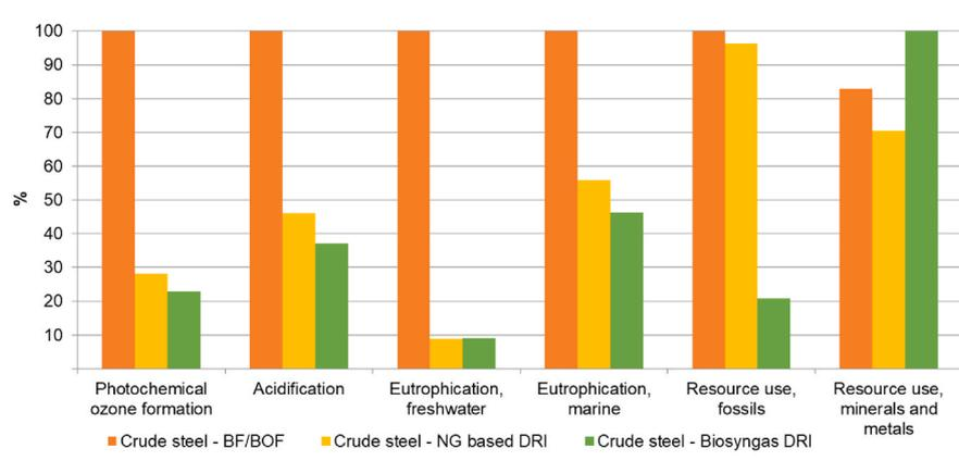
**Fig. 8.** Comparative evaluation of environmental profiles for different iron and steel production technologies. The value of each impact category is normalized and expressed as a percentage. POF = photochemical ozone formation, AP = acidification potential, EP = Eutrophication potential, Resource use.
