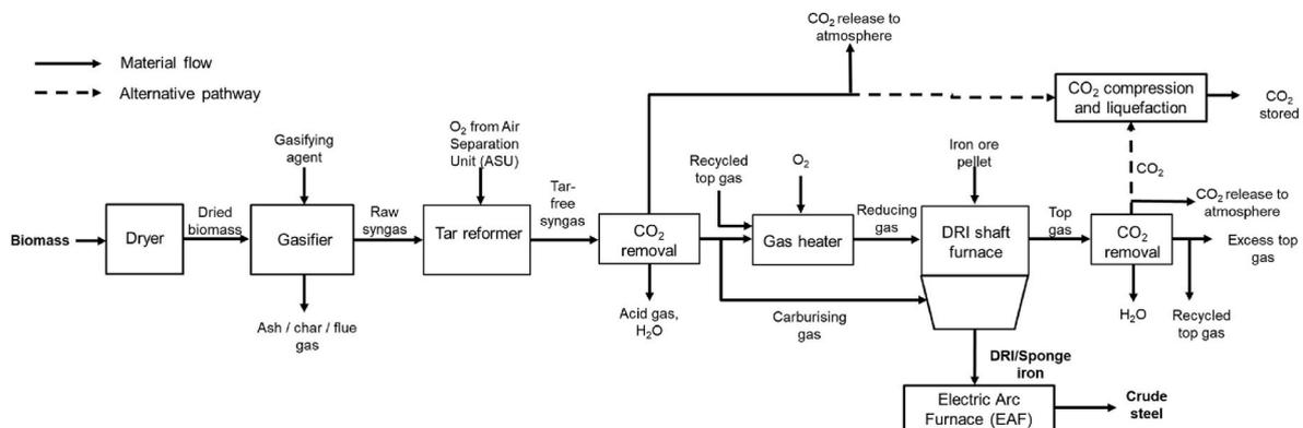
Fig. 1. The general overview of the proposed biosyngas DRI production system. Adapted from (Zaini et al., 2023).
