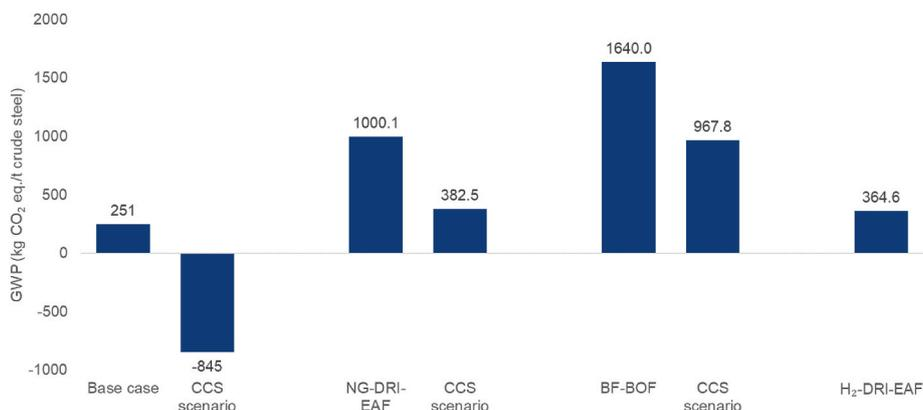
Fig. 7. Comparative evaluation of GWP of different iron and steel production technologies. Partial CCS is applied to all routes, which covers the capture of pure CO<sub>2</sub> streams from DR shaft furnace or blast furnace gas only, while the emissions from EAF and upstream processes are not captured. For the biosyngas-DRI-EAF route, however, CO<sub>2</sub> from biosyngas (gasifier unit) is also removed, as a part of the process requirement, to achieve optimum quality of the reducing gas.
