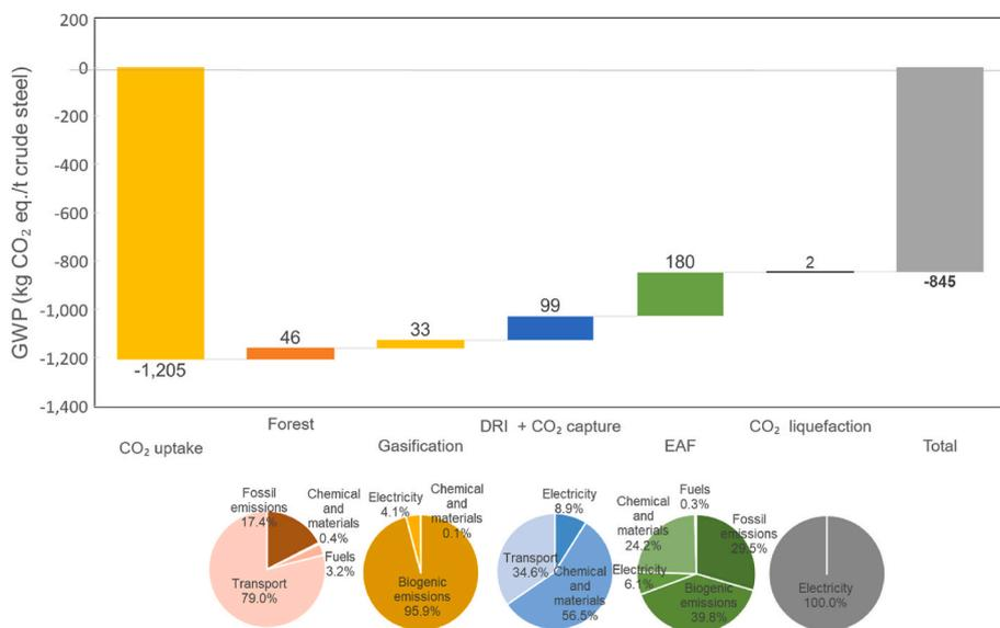
Fig. 6. Cradle-to-gate GWP of crude steel production via biosyngas-DRI-EAF with CO<sub>2</sub> storage. The GWP is presented per subsystem, each includes both direct and indirect emissions. The pie charts show the percentage of emissions contribution.
